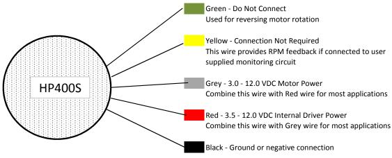
Note: The HP400S will operate on any DC voltage source between 3.5 and 12.0 VDC
